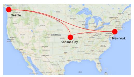
The system is multi-homed in 3 datacenters: New York, Kansas City and Seattle. If one datacenter goes down for some reason, clients will automatically reconnect to the other two (this is an already-provided feature), and the system must continue functioning. The system must also recover from this failure.
